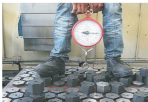
Checking pulling force of chuc
